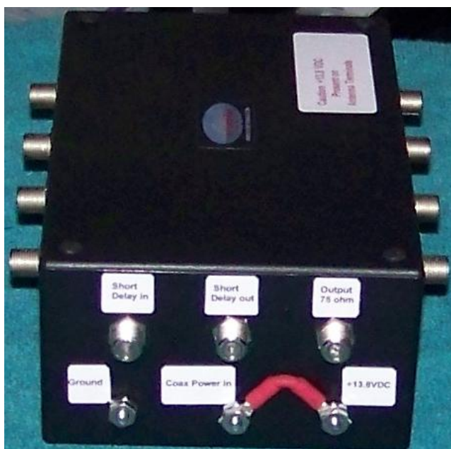
Short Delay Cable and Power View
