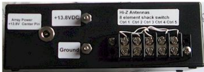
Rear View – Shack Switch
