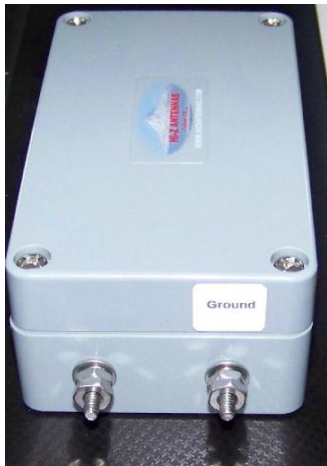
Terminals to Ground and Vertical
