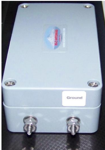
Terminals to Ground and Vertical
