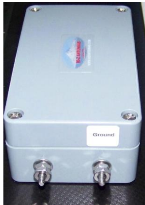
Terminals to Ground and Vertical
