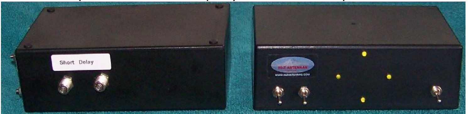
Hi-Z 2, Hi-Z 2-3 Phase controller –left and Shack Switch - right
