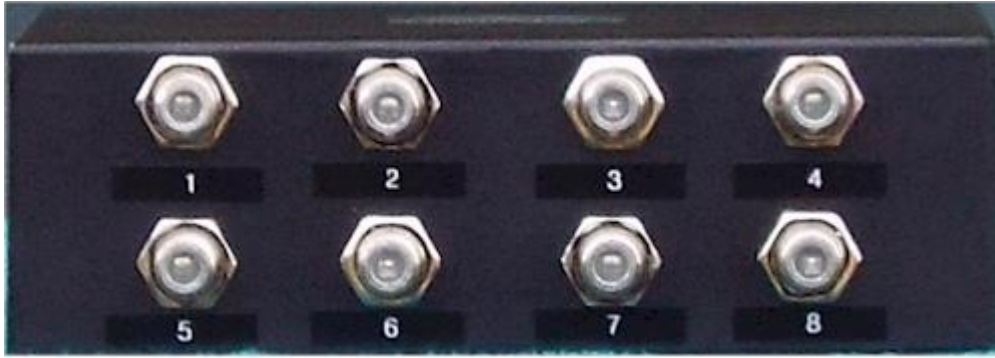
Front Panel is used to accept the 8 cables to be switched
