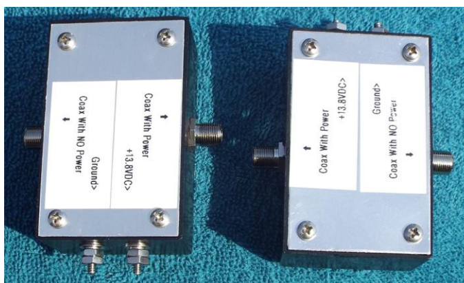
Hi-Z W/L Power Injector – End To End
