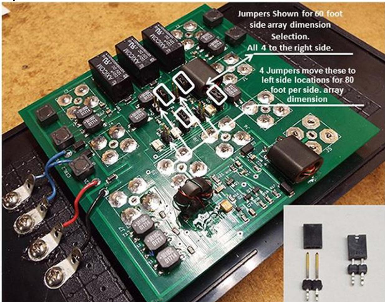
Each little pair of jumpers can be moved from factory setting of 60 foot dimension at the right side to 80 foot settings to the left. Each jumper must remain inline with the relays as seen at the top of the board. It may be pertinent to draw a simple sketch of the pin positions before attempting to move the jumpers if the user is not familiar with these type pin header connectors. All 4 pairs must be moved at the same time in order for the array to work properly.
