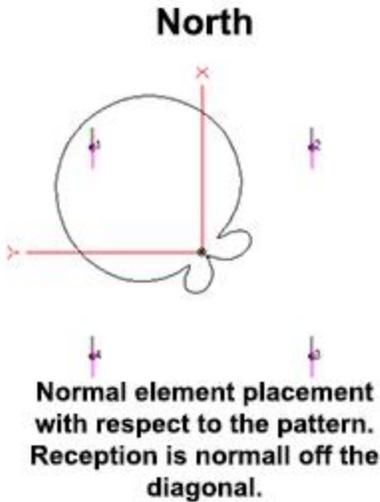
The receiving elements can be placed at 60 or 80 feet per side dimension depending on the user's needs. The elements are placed in a square configuration. The elements need to maintain their equidistant symmetry. The array can be directionally offset if necessary. The HIZ-SS2 and HIZ-SS2-Plus Shack Switch controls can accept offset values however because of the relatively wide pattern an offset would not normally be required with this array.
