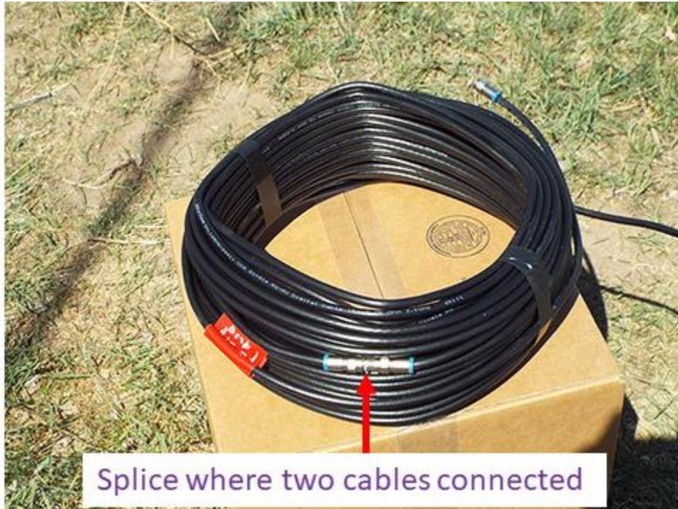
Splice where two cables connected
