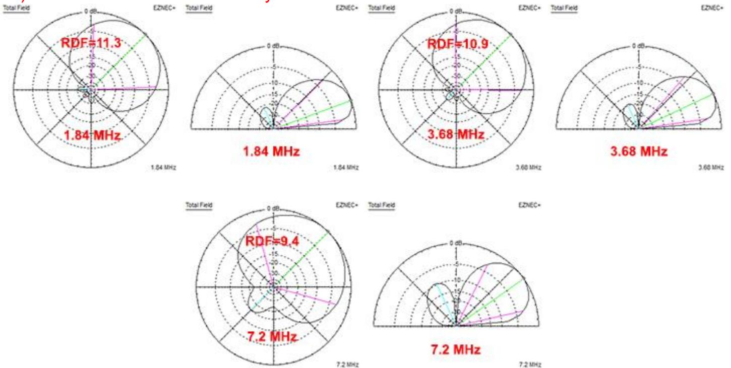
**60 Foot per Side.** One customer adjusted pair of delay cables of 40 degrees for the long delay cable and 20 degrees for the short delay at 1.84 MHz (Max RDF mode) with customer modified delay cables.
