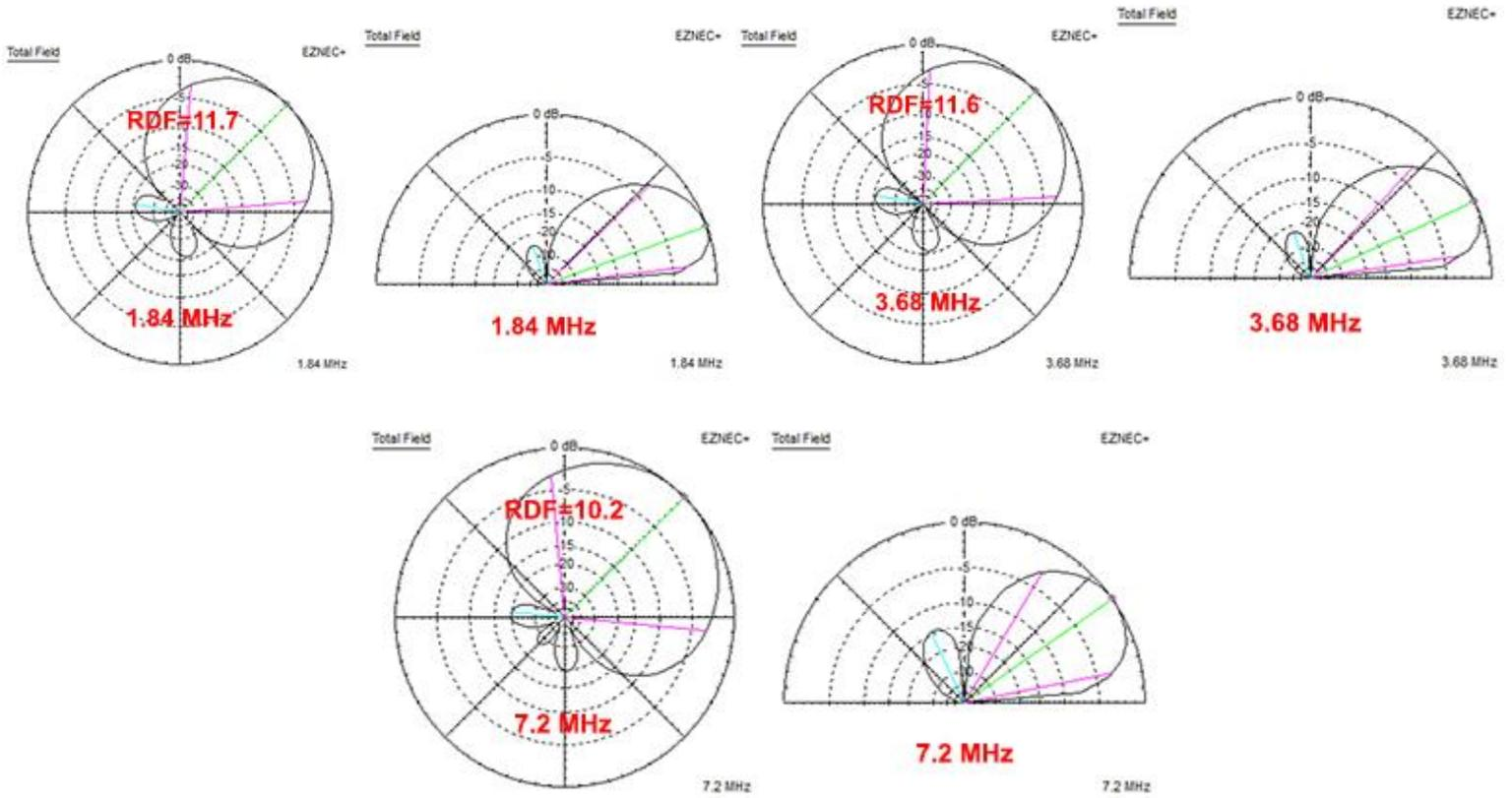
**60 Foot per Side.** One customer adjusted pair of delay cables of 70 degrees for the long delay cable and 35 degrees for the short delay cable at 1.84 MHz (Max Front to Back mode) with customer modified delay cables.
